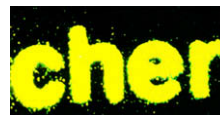
Figure 6. Imaging technique by irradiation ( \lambda \geq 320 nm, T = 40 °C) of an isotropic mixture (E,E) - 1f / (E,Z) - 1f (black area) through a mask. Polarization microscopy shows the birefringent areas, where the S_A phase was photochemically induced.
